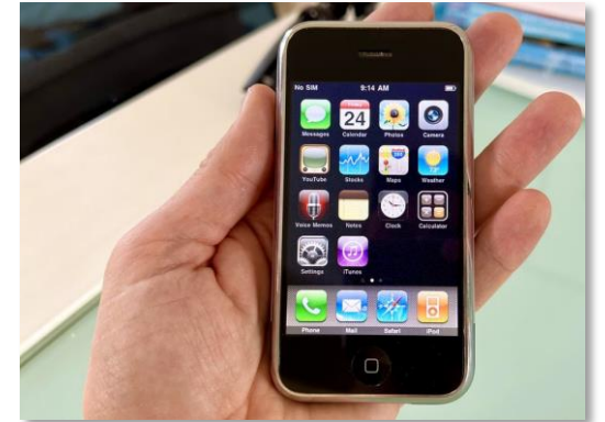
Apple iPhone (Internet Phone) with Samsung S5L8900 SoC, featuring a single core ARMv11 32-bit CPU, 2007
